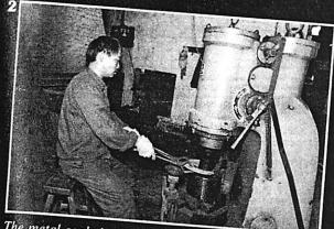
The metal cools in the molds quickly. The cooled castings are then removed and go on to the next step, shown here. Unlike other manufacturing processes that roll the metal out, the Chinese still use the timeless process of hammering the metal to the desired thickness, giving the instrument its "soul." Assisted today with machine hammers at this initial stage, the process itself is patterned after the century-old methods.
